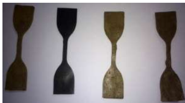
Fig. 1. Cured samples from left, CIIR/NR, CIIR/NR-graphite, CIIR/NR-graphen oxide, CIIR/NR-C 15A
